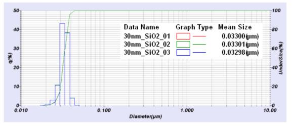
Fig. 3 Comparison of particle size distribution of colloidal silica (30 nm) after centrifugal concentration
