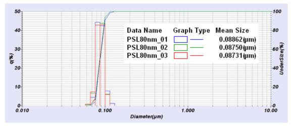
Fig. 4 Comparison of particle size distribution of PSL (80 nm) after centrifugal concentration
