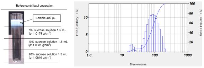
Fig. 1 Sample before centrifugal separation
