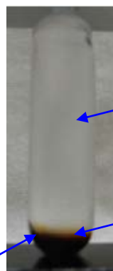
Precipitated Ge particles
