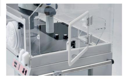
Comfortable, Full-Flat working area with embedded glass warmer and microscope illumination control can be fitted with most of the stereo microscopes available in the market
