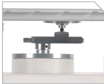
Manual adjustment of rotational angle
