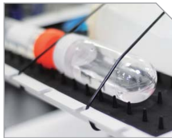
Fastening rubber band tied through the platform edge holes
