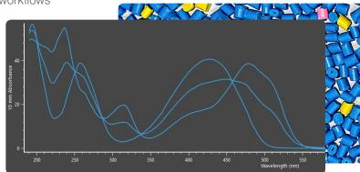
The dyes tartrazine and sunset yellow have overlapping spectra. When combined in a 50:50 solution, only one peak is present. The NanoDrop QC Software runs chemometric algorithms on the instrument and immediately reports component information.
