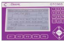
Intuitive user-friendly interface facilitates manual selection of different temperatures in each of the 4x4-well zones, for full user control during PCR optimisation.
