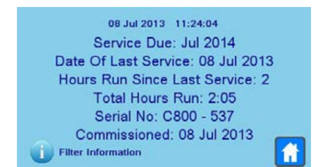
Full information screen with: next and last service date, hours run total and since last service, serial number, commissioning date, current time and date
