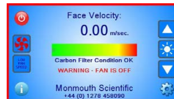
Error screen with warning and audible alarm* - red border indicates unsafe for use
