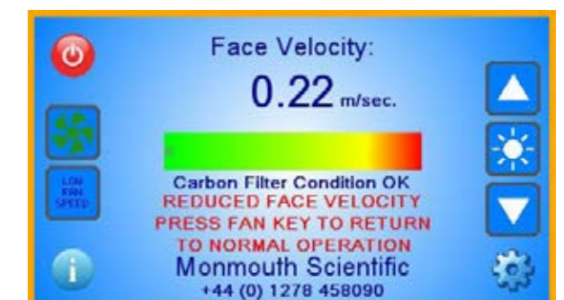
Reduced fan speed operation – yellow border indicates caution
