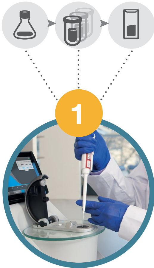
Pipette sample directly onto the pedestal
