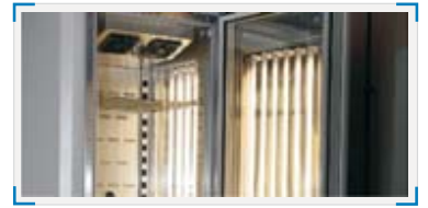
FIT DS - Climatic chambers with lamps installed in the door and side walls
